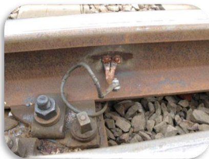
Highly flexible Connectors, Rail bonds, Jumper bonds, Extension bonds etc
