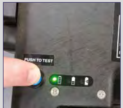
Battery status indicator Green | Amber | Red
