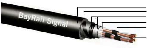
Outer sheath: PE, black Steel tape armouring Al-laminated sheath: PE, black plastic foil Core insulation: PE twisted to a quad
