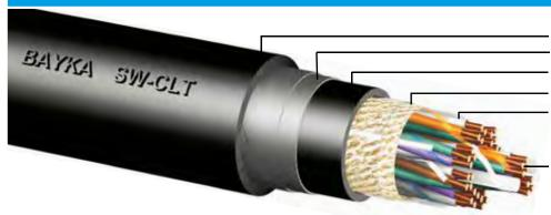
Outer sheath, black Steel tape armouring Inner sheath Core covering Core insulation: PE,
