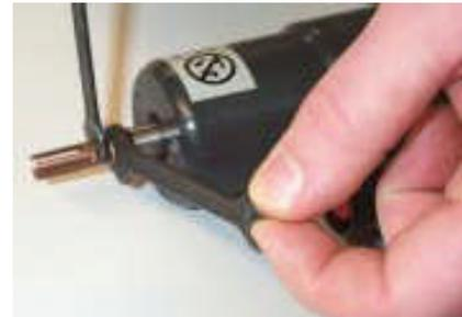
Make sure that pinholder is tight to the gun, use spanners as the figure shows. Otherwise a spark can destroy the axle.
