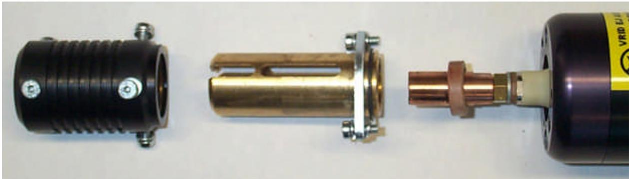
Check that the carbon don't go too loose in the electrode holder, when it does push together with your fingers. Otherwise you can have a contact fault or a spark can arise.
