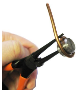
SnakeBite®, pinbrazing without cable lug
