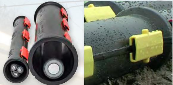
The extremely strong Divisible pipe, Protectus consist of two halves that is easily locked safely with side-locks in different colors for different cable types. Protectus are made of recycled polypropylene and can be reused many times. After its lifetime it's 100% recyclable. Available in lengths of 1 meter and in 4 diameters (Ø 60/110/160/217 mm).
