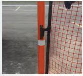
Hook Rapid Link Grip (RLG) to end post lock out handles.
