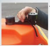
• Remove bungie from cartridge crank handle.
