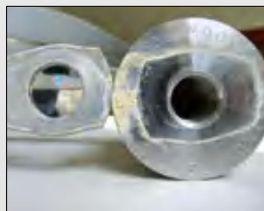
WEB 0 and cable lug after salt spray test
